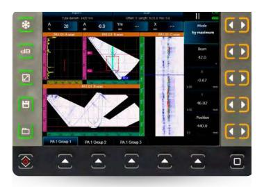
**Weld image on the S-Scan and B-scan based on true beam path** gives the operator easy understanding of defect location and geometry in the object.
